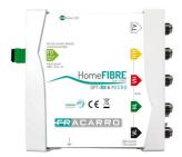
The **OPT OPT-RX 4 MICRO** receiver converts the input optical signal to coaxial signal available on the 4 satellite polarities (VL, HL, VH, HH) and an independent TV output available on the dedicated coaxial connector. The receiver can be powered directly from the output polarities. The product has a multifunctional green LED that provides the installer with various information:
