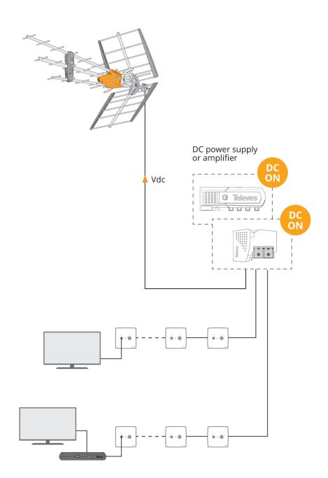
BOSS activation by means of a power supply unit or an amplifier.
